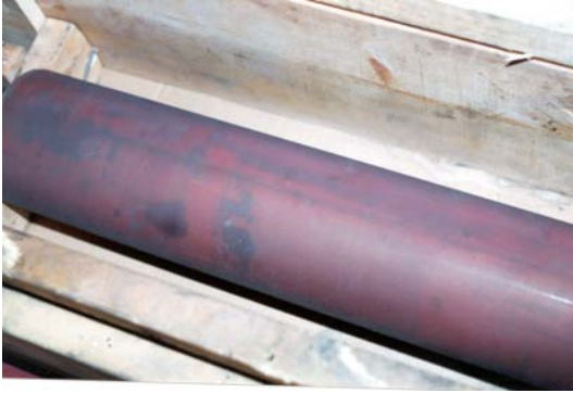
As ink resins harden in the cells, they may trap some pigment causing a visible tint to the roll surface.
